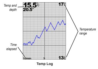
The temperature appears along the right side, and the time elapsed appears along the bottom. The graph scrolls to the left as information is received
